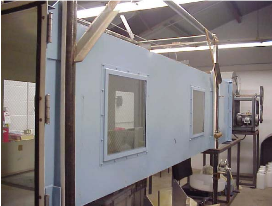
Figure 2-1. MRI Flow Tunnel Test Chamber
