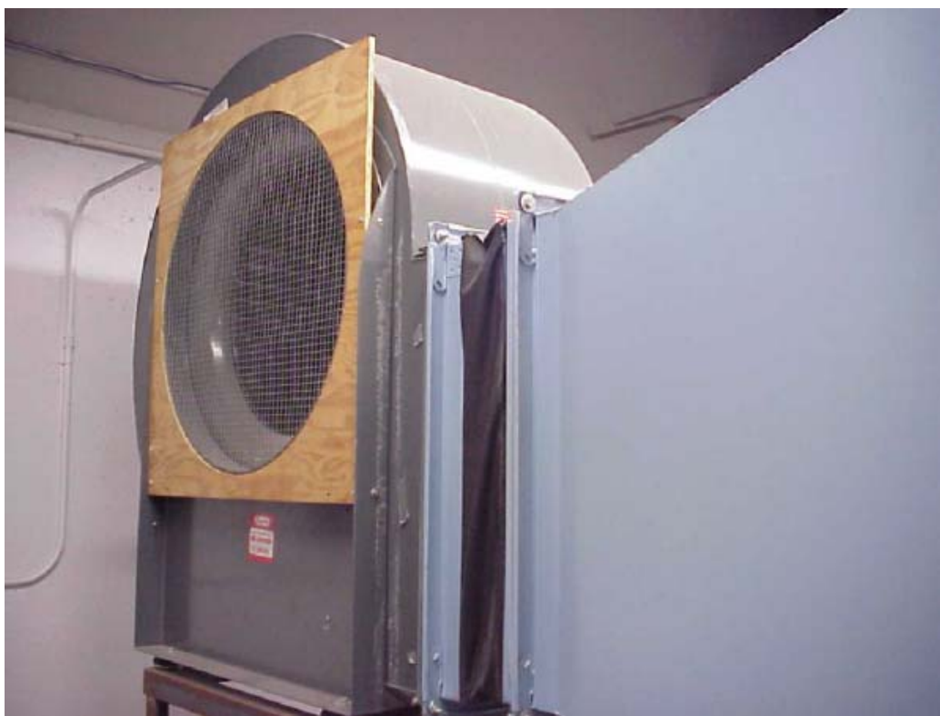
Figure 2-2. Inlet to Test Chamber Blower for Push-Through Operation
