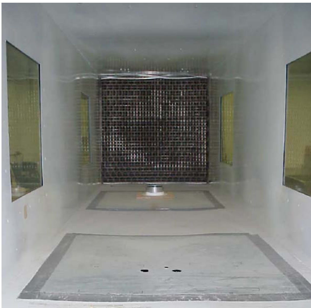
Figure 2-4. Test Chamber Interior With Flow Straightener (viewed from downstream exit)
